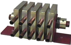
The H-series use liquid cooling to achieve surge duty at very high average power. Our special techniques and materials for disc-to-heat sink interface achieve high power density at a low cost-per-kilowatt.
